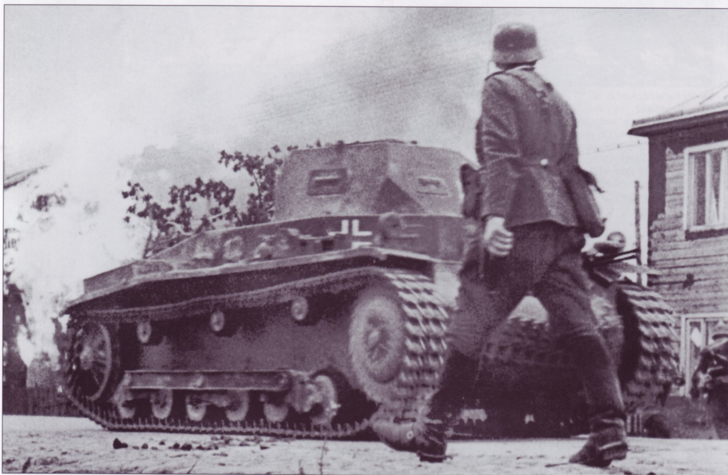
A Pz.Kpfw.II Ausf.a1 of the 3.Panzer-Division rolls into action. The Pz.Kpfw.II Ausf.a1 was the first pre-production model of the Pz.Kpfw.II. Even though only 25 were built in 1936 and supplemented by improved models, it was still in use in September 1939. The Pz.Kpfw.II Ausf.a1 and other pre-production models (Ausf.a2, a3, b) had three pairs of small road wheels attached to a girder-type beam. The Germans committed 3,251 tanks to Poland (losses are in parentheses): Pz.Kpfw.I- 1,445 (89), Pz.Kpfw.II- 1,223 (78), Pz.Kpfw.III- 98 (26), Pz.Kpfw.IV- 211 (19), Pz.Kpfw.38(t)- 59 (6), plus 215 command tanks (losses unknown, possibly included with the basic models) of all types assigned to six Panzer and four light divisions plus a few odd separate units. The light divisions, essentially cavalry arm mechanized formations, would later be reorganized and redesignated Panzer divisions.
