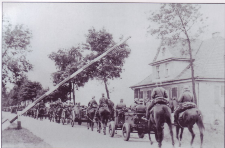
A German artillery battery crosses the frontier beside a Polish customs house with its 10.5cm IFH 18 field howitzers followed by an Hf.7 steel field wagon (Stahlfeldwagen). The latter was an all-metal, rubber-tired utility wagon drawn by four horses. Older-style wooden bed, spoked wooden-wheeled wagons and carts were in much wider use though.
