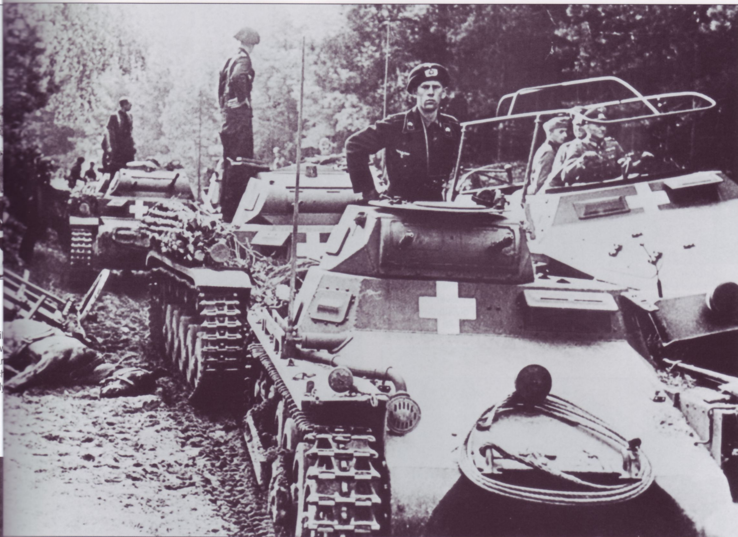
General Heinz Guderian, commanding the 4.Panzer-Division, passes a column of light tanks. In the foreground is a Pz.Kpfw.I Ausf.B followed by two Pz.Kpfw.II Ausf.As. Guderian utilized the Sd.Kfz.251/6 command vehicle (Befehlswagen) version of the medium rifleman's armor vehicle (mittlerer Schützenpanzerwagen—mSPW) complete with long-range radios and an Enigma cryptographic device.
