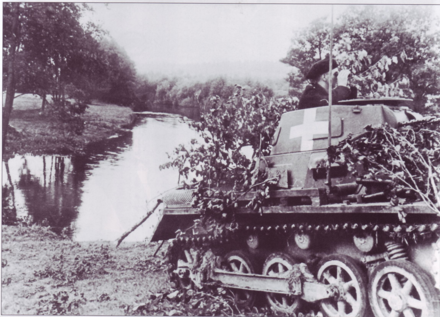
The commander of a Pz.Kpfw.I Aüs.f.A (four road wheels, other types had five and a lengthened hull) observes his route for enemy activity before advancing further. Foliage attached to a tank provides little camouflage if moving, but if halted it offers some degree of concealment from distant ground and air observers. MG.34 machine guns installed in Pz.Kpfw.Is habitually lacked flash suppressors.
