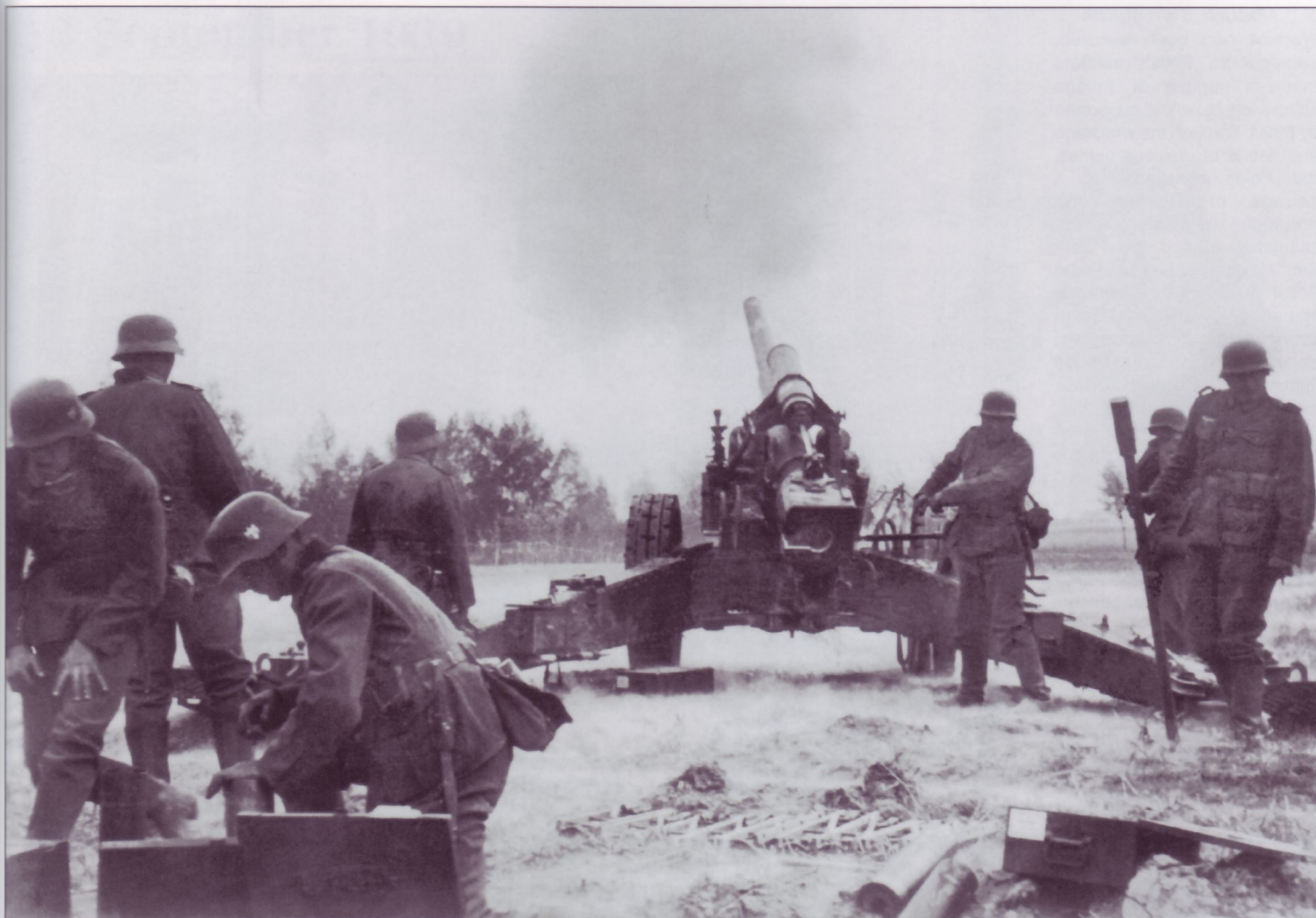
A 10cm sK.18 heavy gun pounds enemy positions somewhere in central Poland. Some divisional 15cm howitzer battalions also possessed a four-gun 10cm (actually 105mm) battery for counterbattery employment. It was mounted on the same carriage as the 15cm sFH 18, but had a much longer barrel. The 10cm had a range of 19,075 meters, almost 6,000 meters further than the companion 15cm howitzer.
